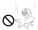
◎ Do not manually pan and tilt the USB Camera when it is rotating by electrical power.
